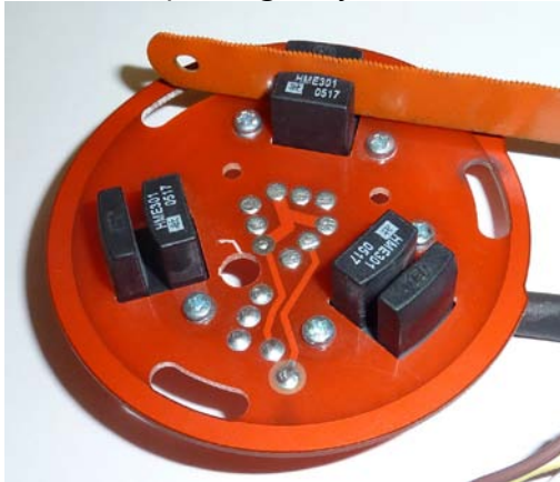
Testing the sensor with a steel blade
