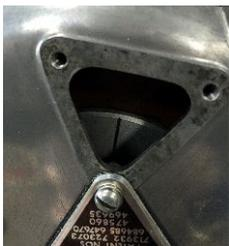
If the plunger tool is not available simply rotate the crank backwards from TDC until the FIRST timing mark lines up with the pointer as shown. In most cases this will be the "B" mark. The crank should now be lined up at 38 degrees BTDC ready for the installation.
