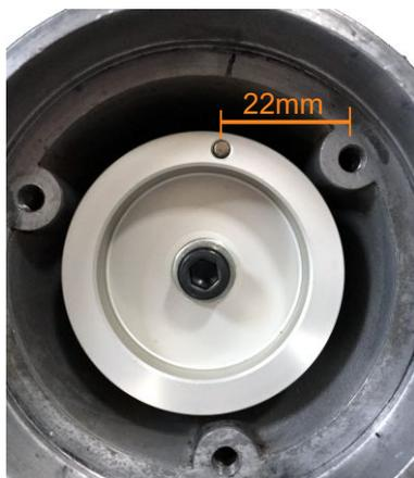
Install the trigger rotor as shown above 22mm centre to centre from the magnet to the bolt hole. The socket head screw provided is the correct 1/4 UNF thread - it should go in easily. If it bottoms you will need to shorten it - don't force it !
