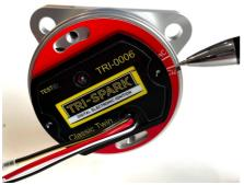
Loosely install the stator unit in the housing so that the holes for the pillar bolts are in the centre of the adjustment slots as shown here. Mark the housing with a pen as shown next to the text 'CW' on the right edge and then remove the stator unit.
