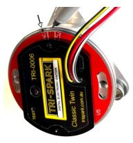
Loosely install the stator unit in the housing so that the holes for the pillar bolts are in the centre of the adjustment slots as shown here. Mark the housing with a pen next to the letters 'AC' and then remove the stator unit.
