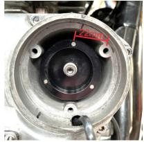
available simple rotate the crank backwards from TDC until the FIRST timing mark lines up with the pointer. In most cases this will be the "B" mark. The crank should now be lined up at 38 degrees BTDC ready for the installation.
